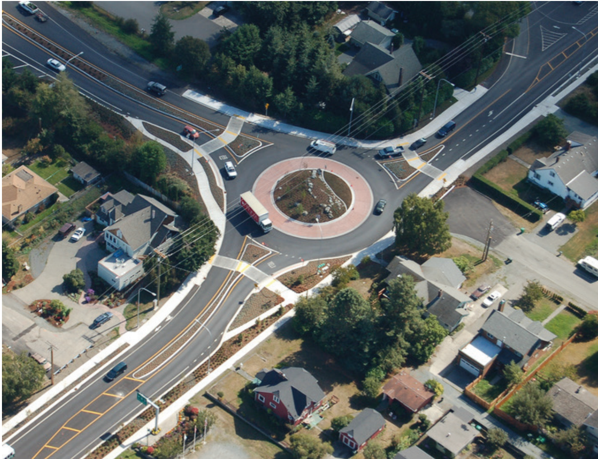
Example of a Roundabout LINK
