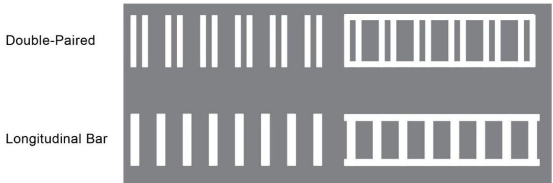
Figure 10: Recommended HVC Marking Styles for All Crosswalks.
